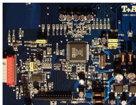
This board features four inputs for Scart, YUV, S-Video and Video, and once the conversion process is complete, the original analogue picture data is present in digital form at the very highest quality, ready for further processing. The data can now be passed to the video processing section in exactly the same way as the signal coming from the HDMI
