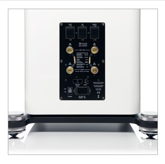
All SOLITAIRE® models are fitted with level adjusters for the mid-range and electrostatic drivers. Instead of modifying the frequency response, the adjusters alter the loudness level of the drive units. This makes it possible to fine-tune each loudspeaker individually to suit its position in the room, thereby largely eliminating problems associated with their location.
