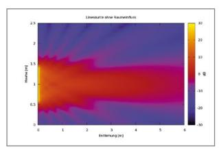
The graph alongside shows the radiation behaviour of a Line Source - such as the electrostatic driver used in the CWT 1000-8 SE - without the influence of a room. Interference effects produce a homogeneous, cylindrical, axial sound dispersion pattern in front of the loudspeaker, whose intensity does not diminish even over quite a long distance.
