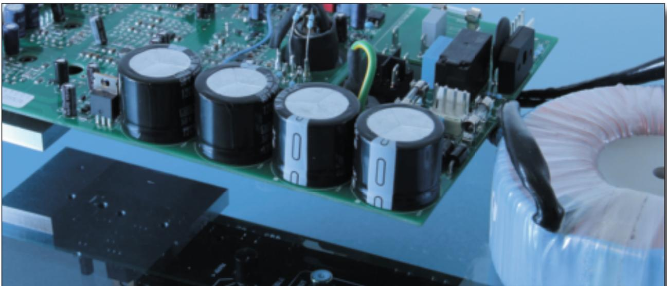
The main circuit board of the active unit accommodates the input section, the active cross-over unit, the output stages and the sophisticated mains section with stabilised multi-voltage power supply. The generously dimensioned, hum-free toroidal transformer features a high overload reserve, and is mounted separately on the base plate on absorbers.
