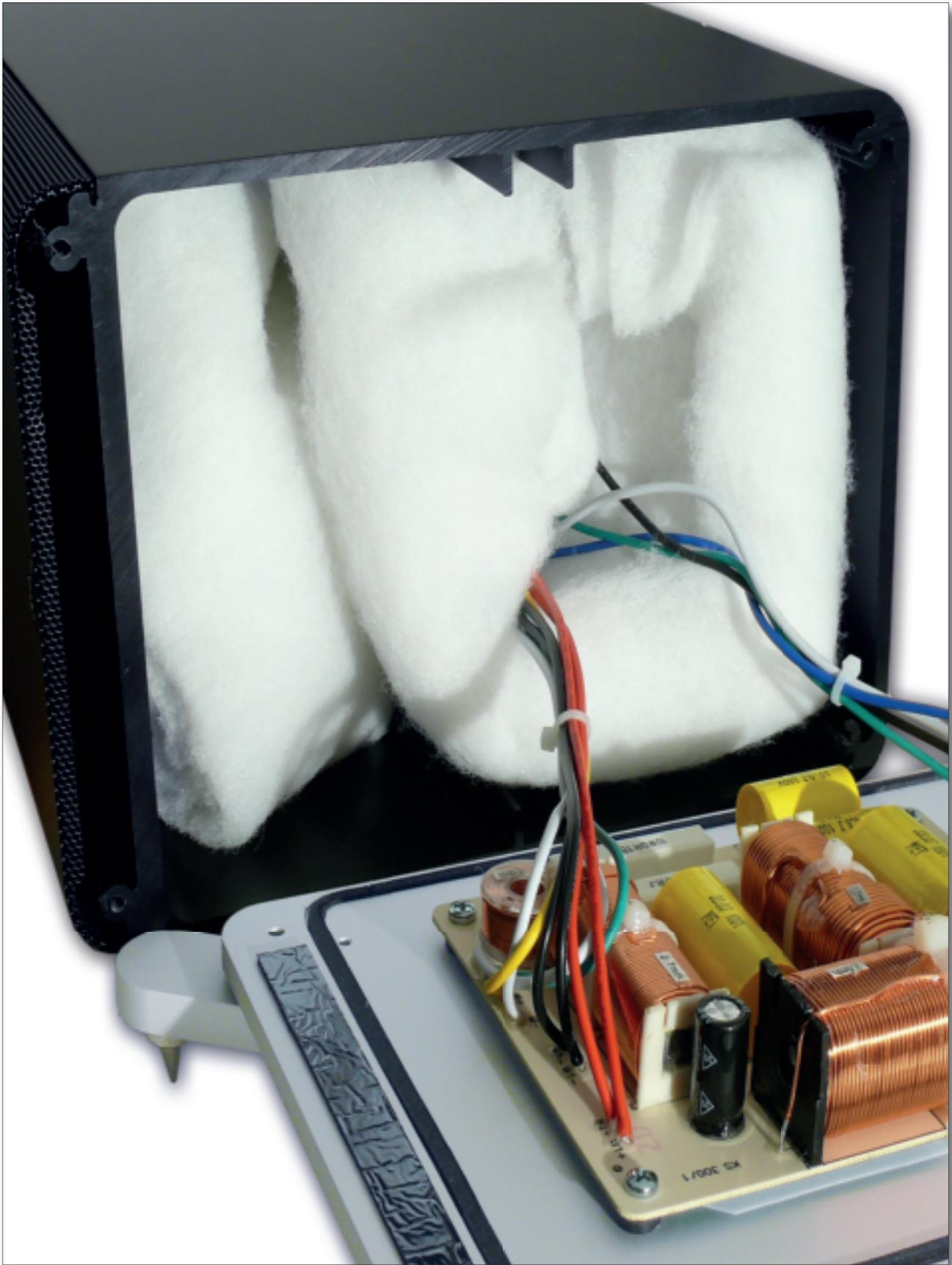
Single-piece pressing: the solid aluminium cabinet of the KS 300, KS ACTIVE and KS 350. The manufacturing process incorporates integral supplementary stiffening ribs, guides for internal bracing, grille mountings and screw channels. This type of large, heavy, complex extrusion can only be produced to the required standard of precision using the latest technologically advanced extrusion machines.
