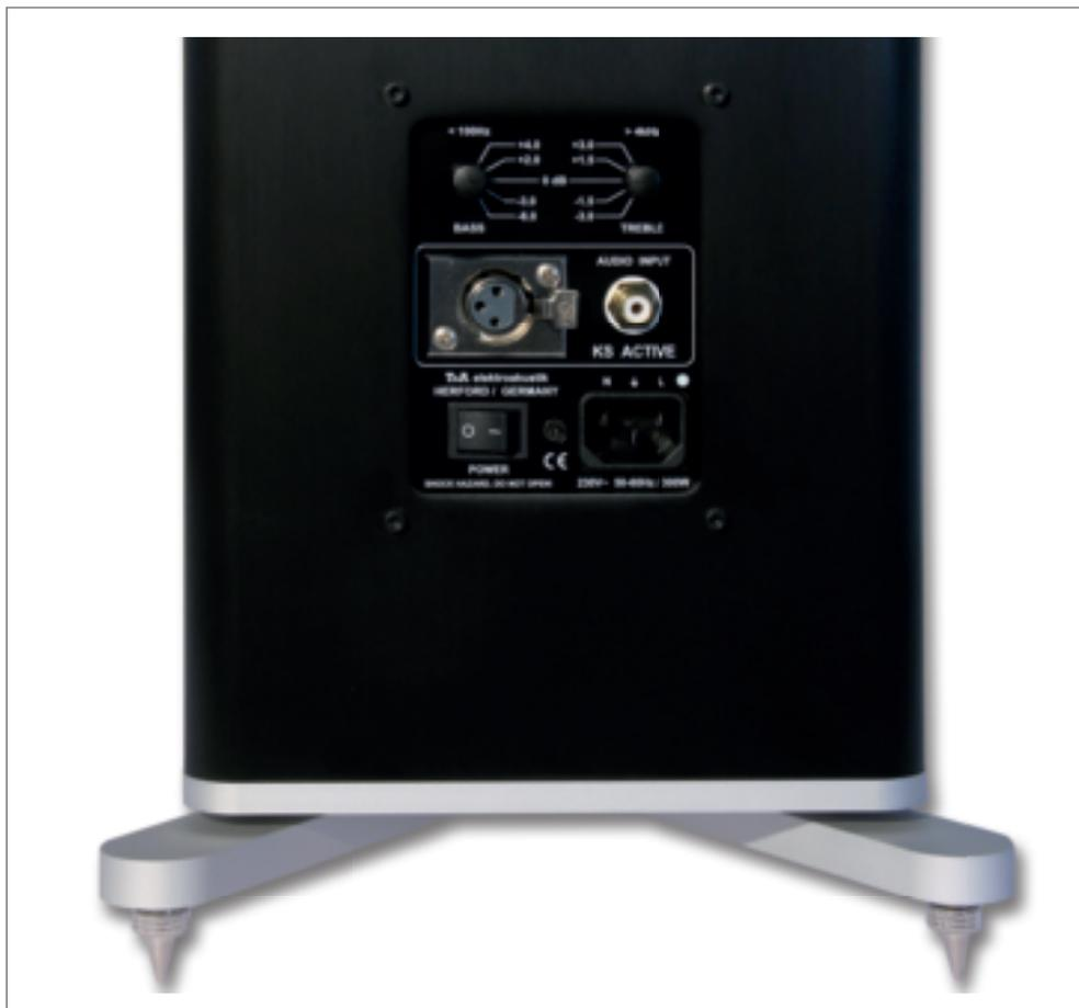
The active electronic unit forms a self-contained assembly which is mounted on the back panel of the loud-speaker cabinet. A metal plate carries the double-sided main circuit board bearing the XLR and Cinch (RCA) inputs, the mains power socket, the separate mains switch and the switches for position and room equalization. The KS ACTIVE switches itself on automatically when a music signal is present, or by a DC trigger voltage at the Cinch (RCA) socket (Caruso).
