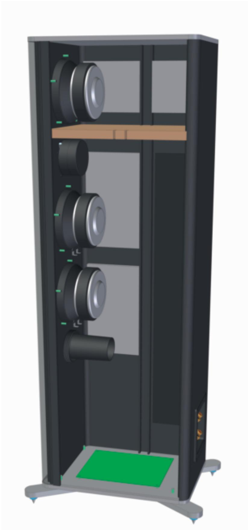
This CAD drawing shows the internal construction of the KS 300: the mid-range unit is housed in its own airtight chamber, which is separated from the rest of the cabinet by an MDF partition. This component, in conjunction with additional plates, damps the cabinet walls extremely effectively. A relatively large internal volume is available to the two bass units, which can therefore be tuned to operate at very low frequencies. A bass port augments the lowest frequencies.
