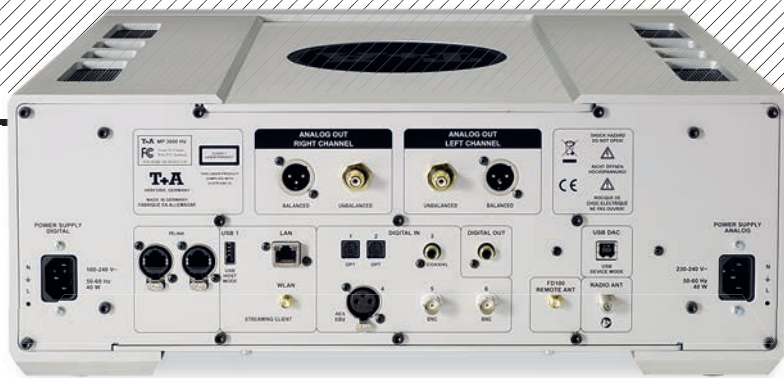
ABOVE: Balanced (XLR) and single-ended (RCA) analogue outs, both fixed, are joined by S/PDIF (RCA, two on BNC and two Toslink), AES/EBU (on XLR), USB 2.0 and wired and wireless Ethernet digital connections. The RF remote connects via an aerial. Note two IEC mains inlets for separate 'digital' and 'analogue' circuit power supplies
