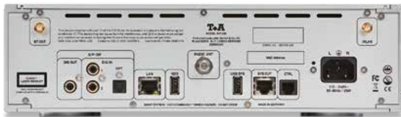
ABOVE: The MP 200 hosts BT, WLAN and FM radio antennas with hardwired LAN, coaxial (2x) and optical digital inputs alongside USB-A for external HDDs. Outputs are on coaxial RCA (S/PDIF) and proprietary SYS Out (RJ45)/USB SYS connections
