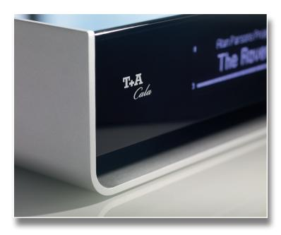
The case is made of solid aluminium, and is produced in a single process using a complex extruding tool. It is then blasted with fine glass beads before being anodised. The internal chassis, on which all the electronic circuitry is mounted, is also made of aluminium, while the front panel and top cover consist of high-gloss acrylic.
