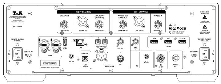
Depending on the version of the PSD 3100 HV, the WLAN antenna and IPA Link connections may be swapped
