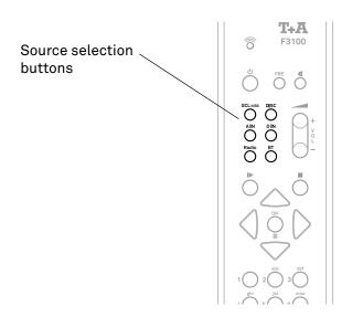
A brief press on these buttons selects the desired source. To simplify the source selection, the sources are grouped by category on one button each. Press the appropriate button repeatedly, if necessary, until the desired source is shown in the PSD 3100 HV display.
