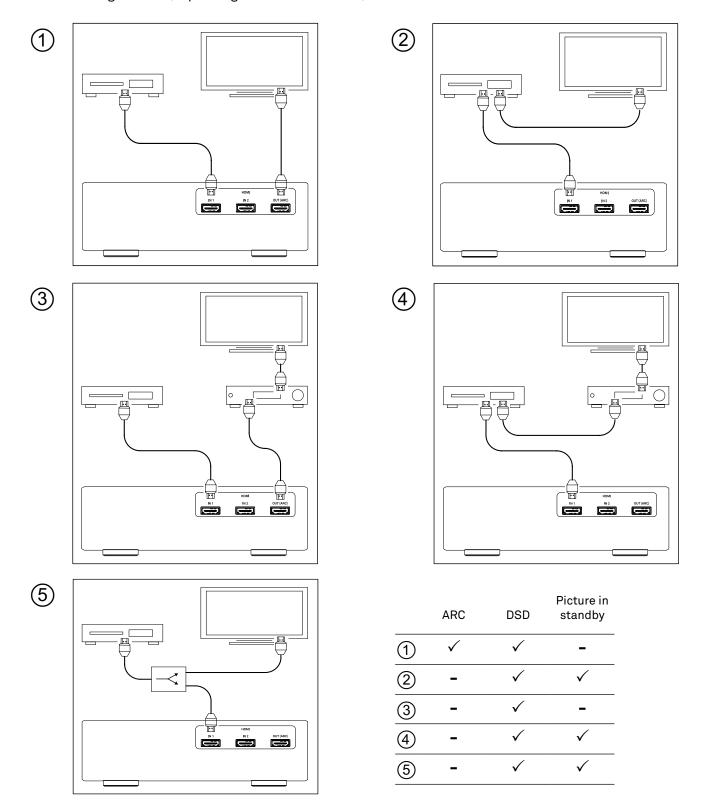
ARC = TV sound via PSD 3100 HV; DSD = DSD playback; Picture playback in standby = playback from source device to TV set while PSD 3100 HV is switched off
