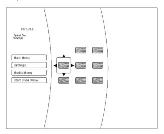
You can now use the menu options on the left-hand side of the screen to select the whole folder as a 'slide show', or select a single picture to be displayed by selecting with the navigation buttons and confirming your choice with the OK button.
