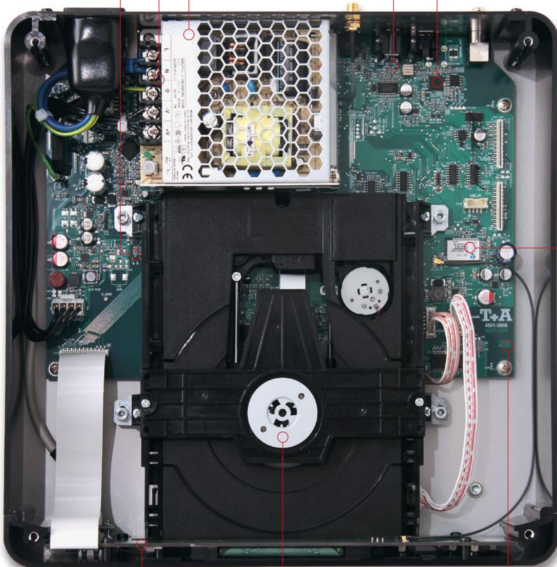
Front Control board with dimmable OLED display and Bluetooth aerial.
