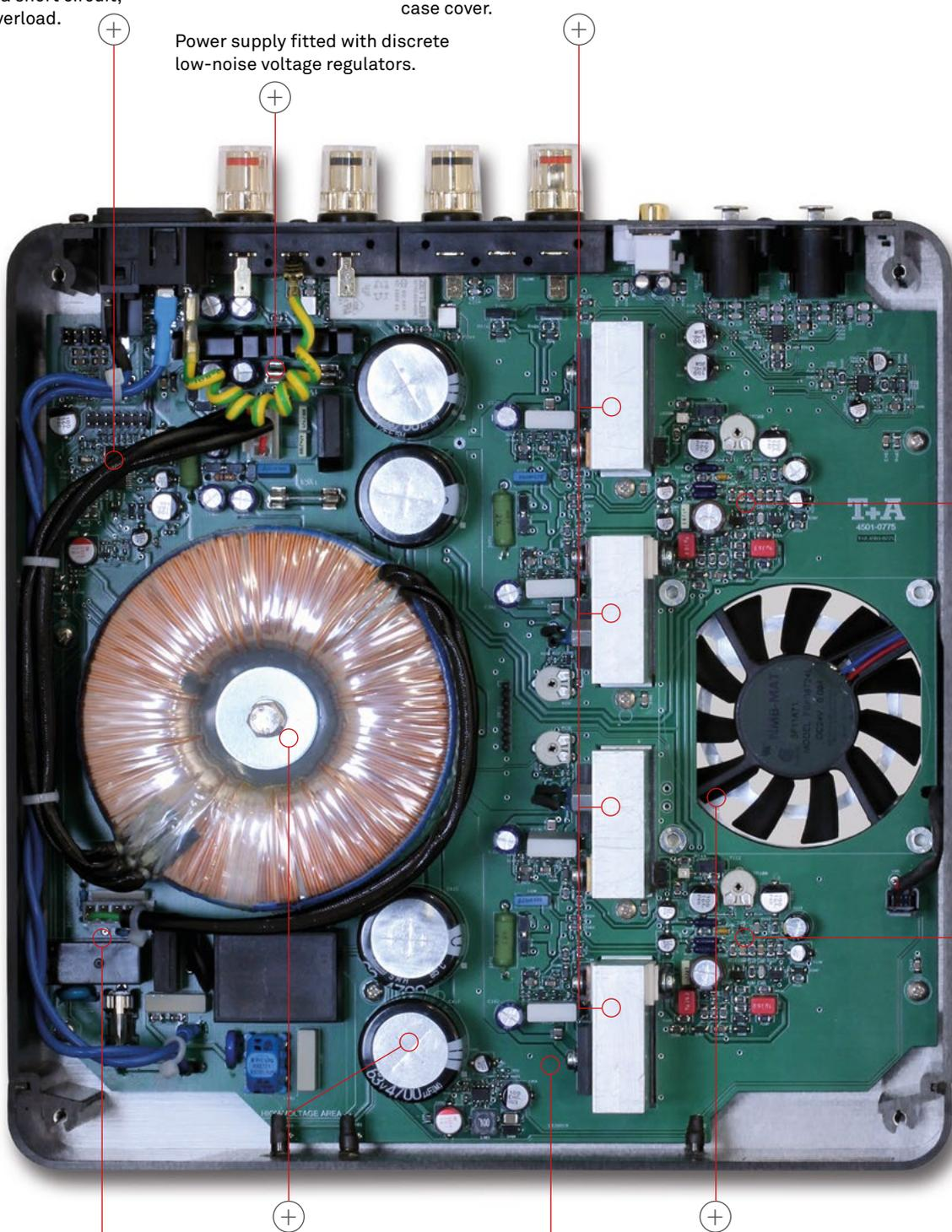
Sophisticated mains filtering to block RF interference and DC voltage.
