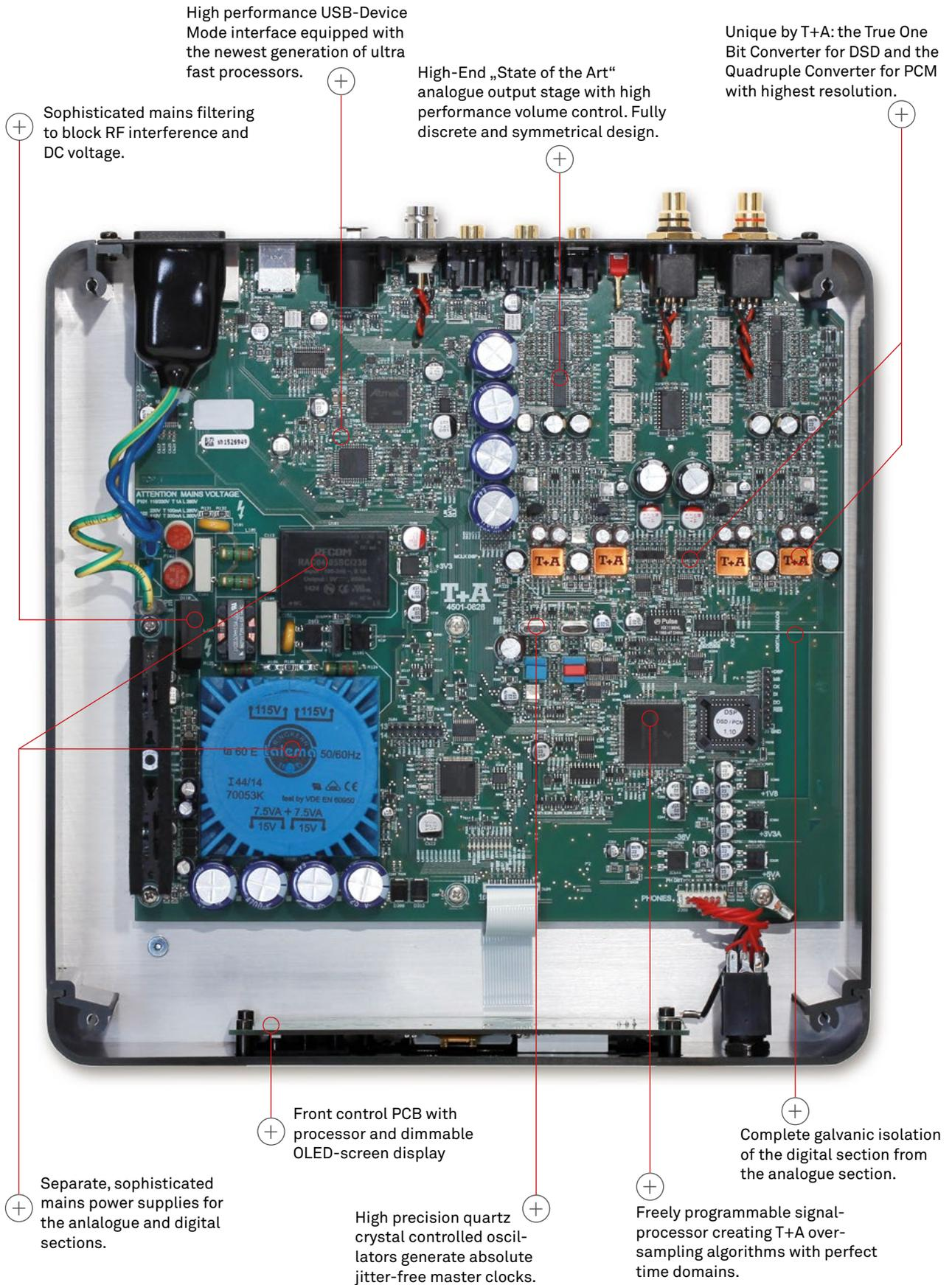
High performance USB-Device Mode interface equipped with the newest generation of ultra fast processors.
