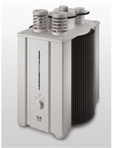
The symmetrical input amplifier is a valve amplifier in a cascode circuit, controlling the High Voltage (HV) Class A J-FET voltage amplifier stage; the amplification factor is 50. This is followed by two separate current amplifiers with an amplification factor of 1 exploiting MOSFET transistors on the input side, and high-performance bi-polar ring emitter transistors on the output side.
