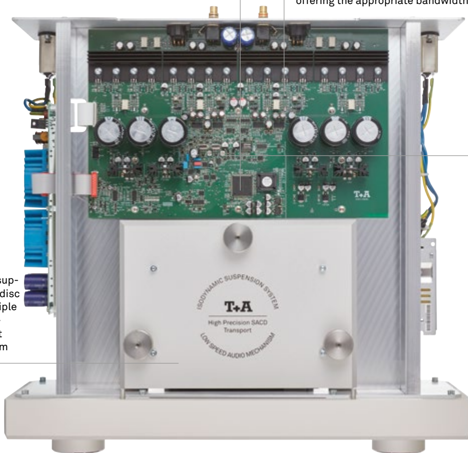
Internal view of the upper case compartment MP 3100 HV
