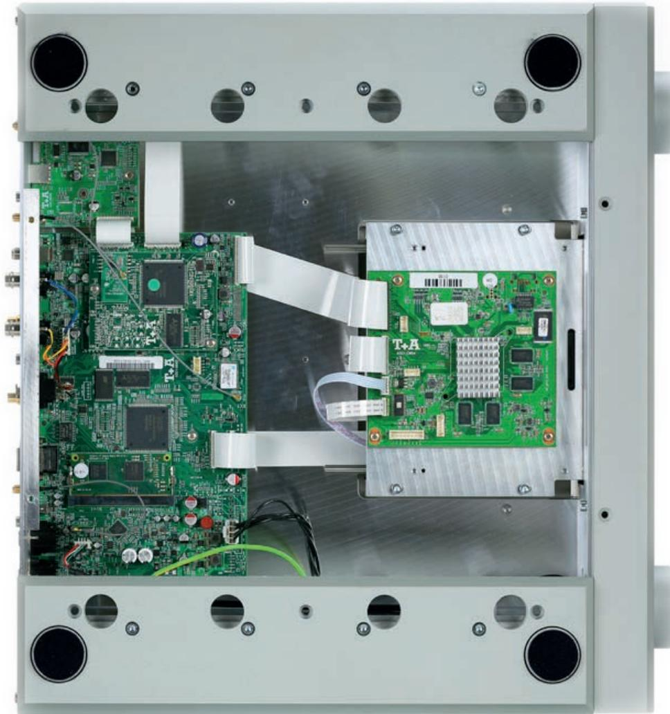
processed by separate converters with independent, completely distinct signal paths. According to head developer Lothar Wiemann, the resulting isolation of the analog and digital parts eliminates any digital interference. The converters themselves are proprietary developments created by the minds at T+A: For DSD signals, the manufacturer relies on its own fully discrete True 1 Bit DSD
