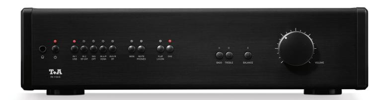
The PA 1100 E provides five high-quality inputs which are selected using gold-contact relays; one of these can be set up as XLR input. It is also possible to upgrade IN4 to a phono input using the PHE MM or PHE MC internal modules (earth terminal present). REC OUT and PRE OUT are available. The heavy-duty loudspeaker terminals are gold-plated and contain no ferro-magnetic metals. Five high-resolution digital inputs are available for connecting external digital sources, typically for playing data
