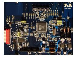
This board features four inputs for Scart, YUV, S-Video and Video, and once the conversion process is complete, the original analogue picture data is present in digital form at the very highest quality, ready for further processing. The data can now be passed to the video processing section in exactly the same way as the signal coming from the HDMI
