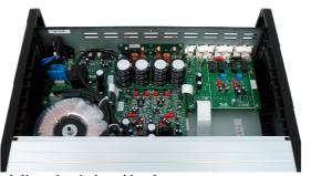
analogue construction. The output stages feature an analogue feedback circuit, which eliminates any problems caused by voltage fluctuations in the mains power supply,
