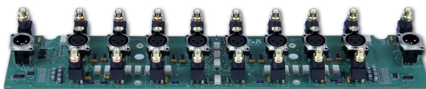
The High-End sockets are soldered directly to the circuit board, and screwed permanently to the aluminium back panel.
