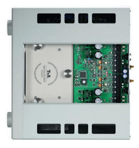
method, digital artifacts such as pre- and post-ringing are excluded. It's well known that to produce optimal playback data needs to be cleansed of the notorious jitter before DCA conversion., so it's not surprising T+A relies on its own concept for jitter elimination. This works in two stages: In the first, the data received is processed and decoded. In the process, a rough pulse is
